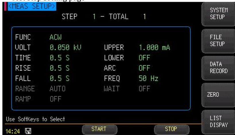
Current step 1-total steps: the step ID of the test plan, the current parameter is the number of steps in the test plan – there are several steps in total
